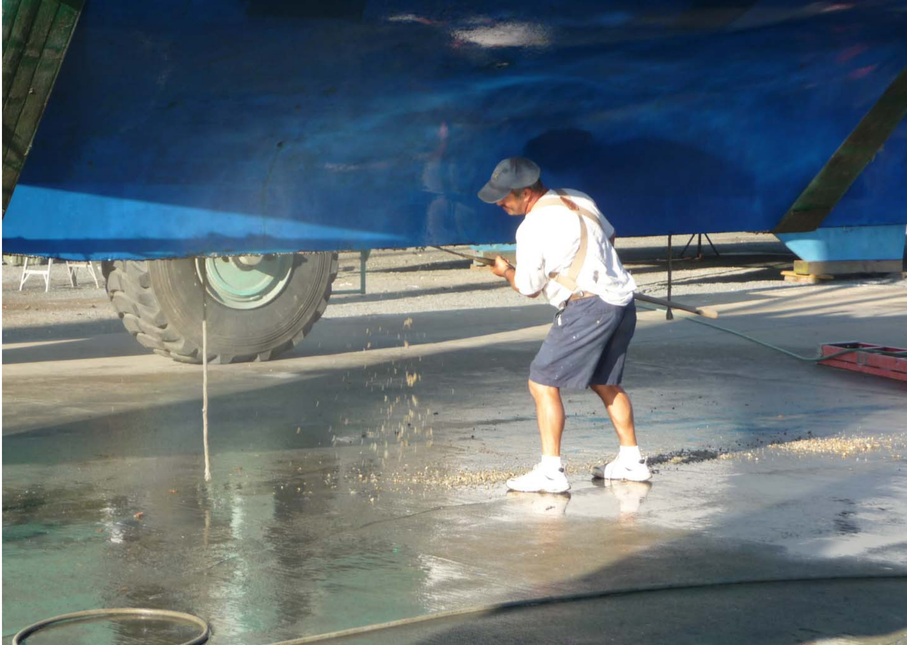
Scraping off the barnacle build up on the stem of the hull & on the centerboard.
