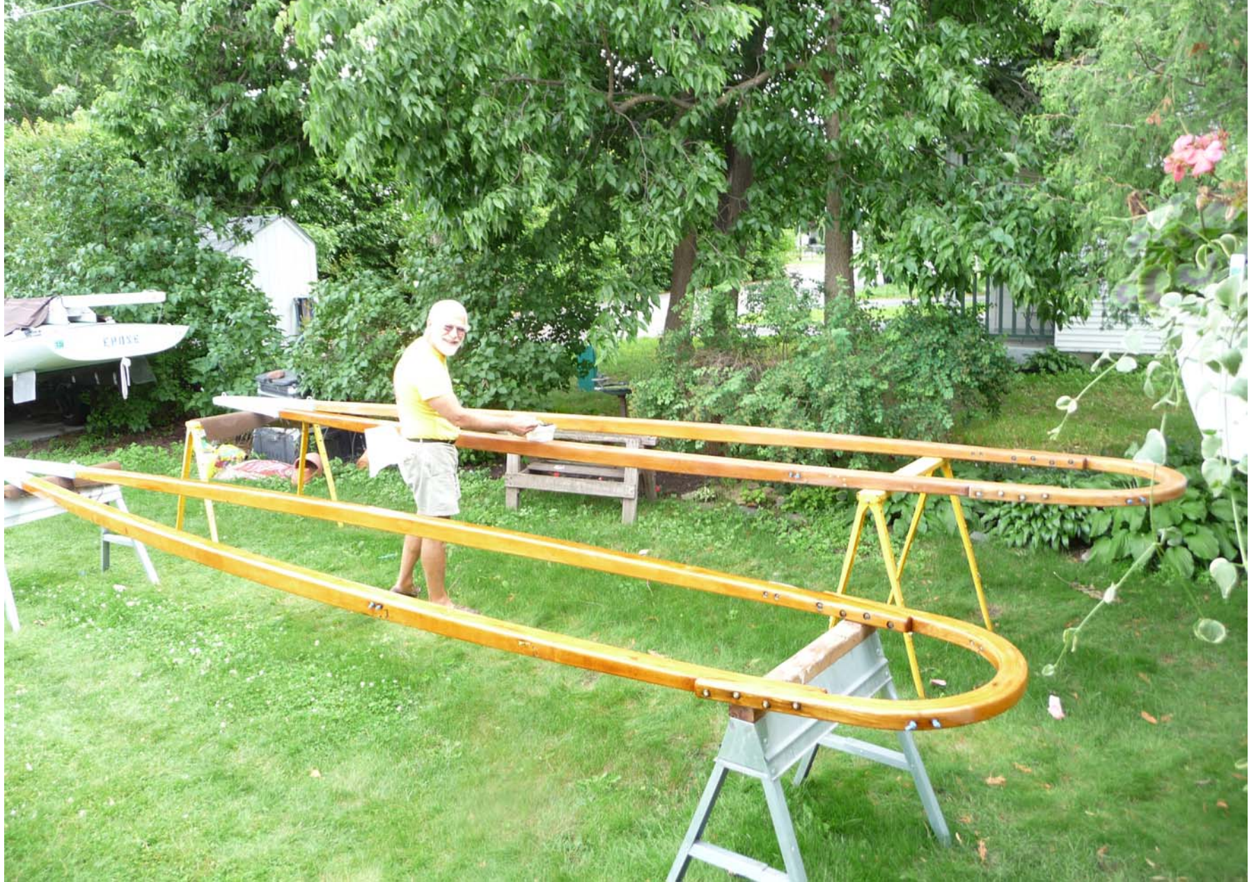
Carl refinishes Running Free's two wishbone booms in our back yard with 10 layers of spar varnish.
