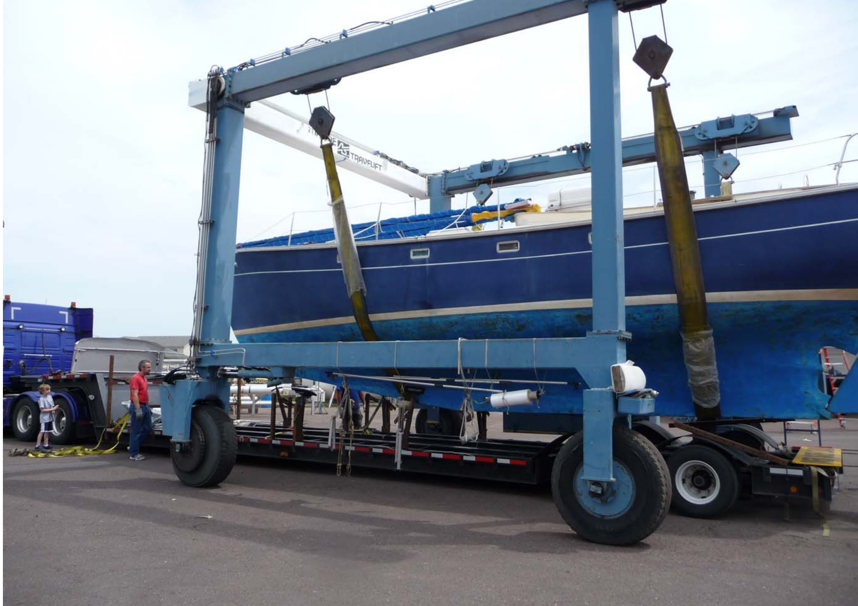
Here the Barker's Island Marina crew uses the Travel Lift to take the boat off the truck trailer.
