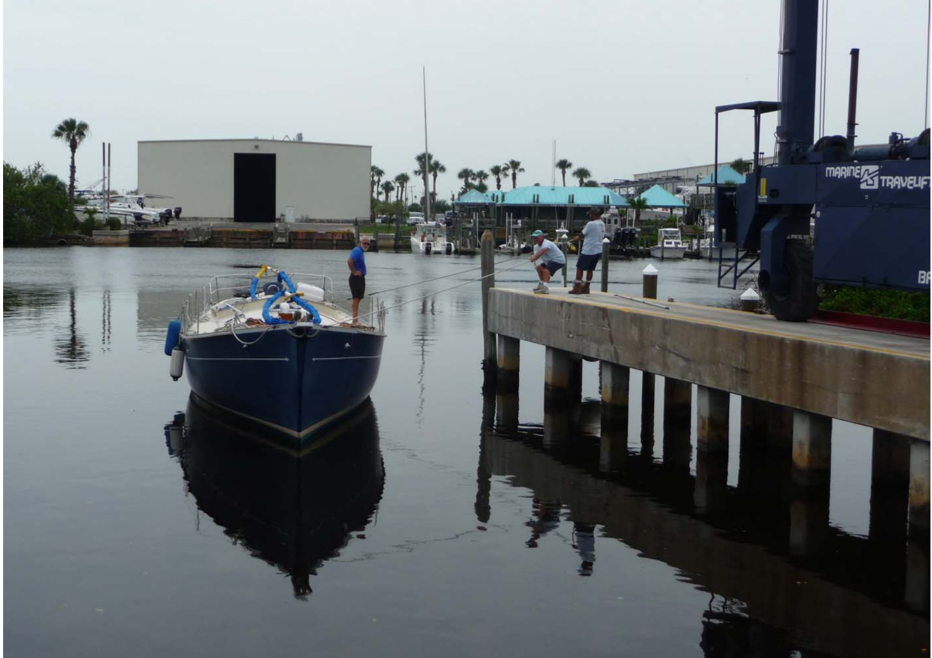
The boat is then warped around into the haul out well.
