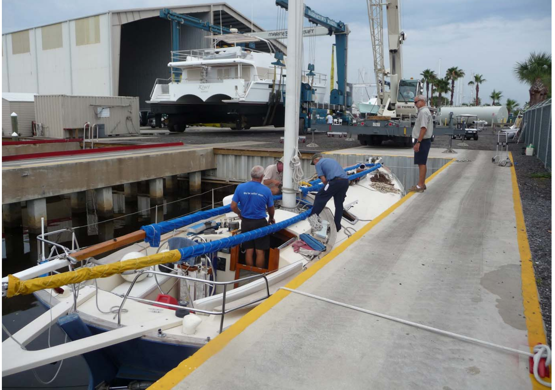
Here the Boat Yard crew are working on getting our mizzen mast out.
