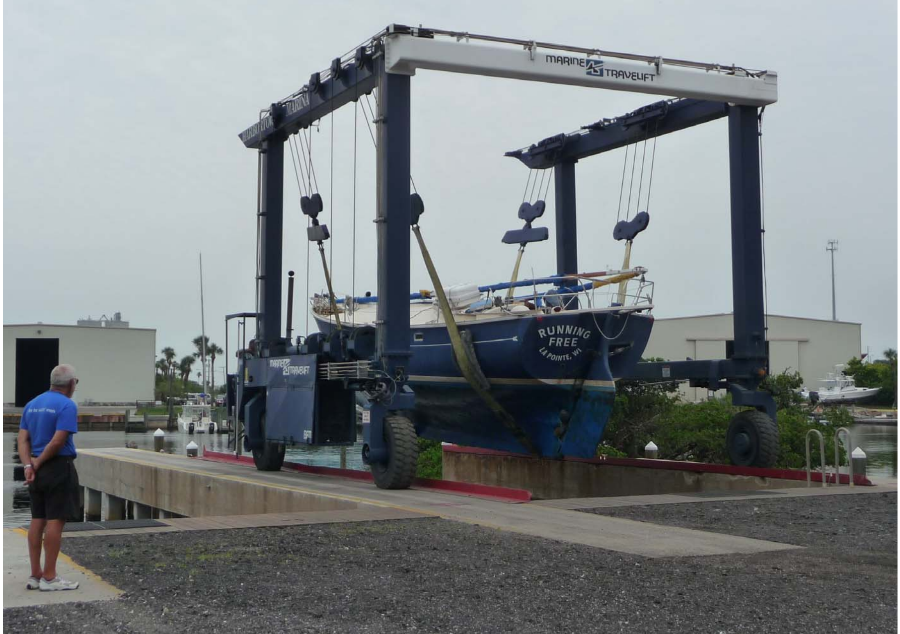
Running Free is lifted out—all 10+ tons.
