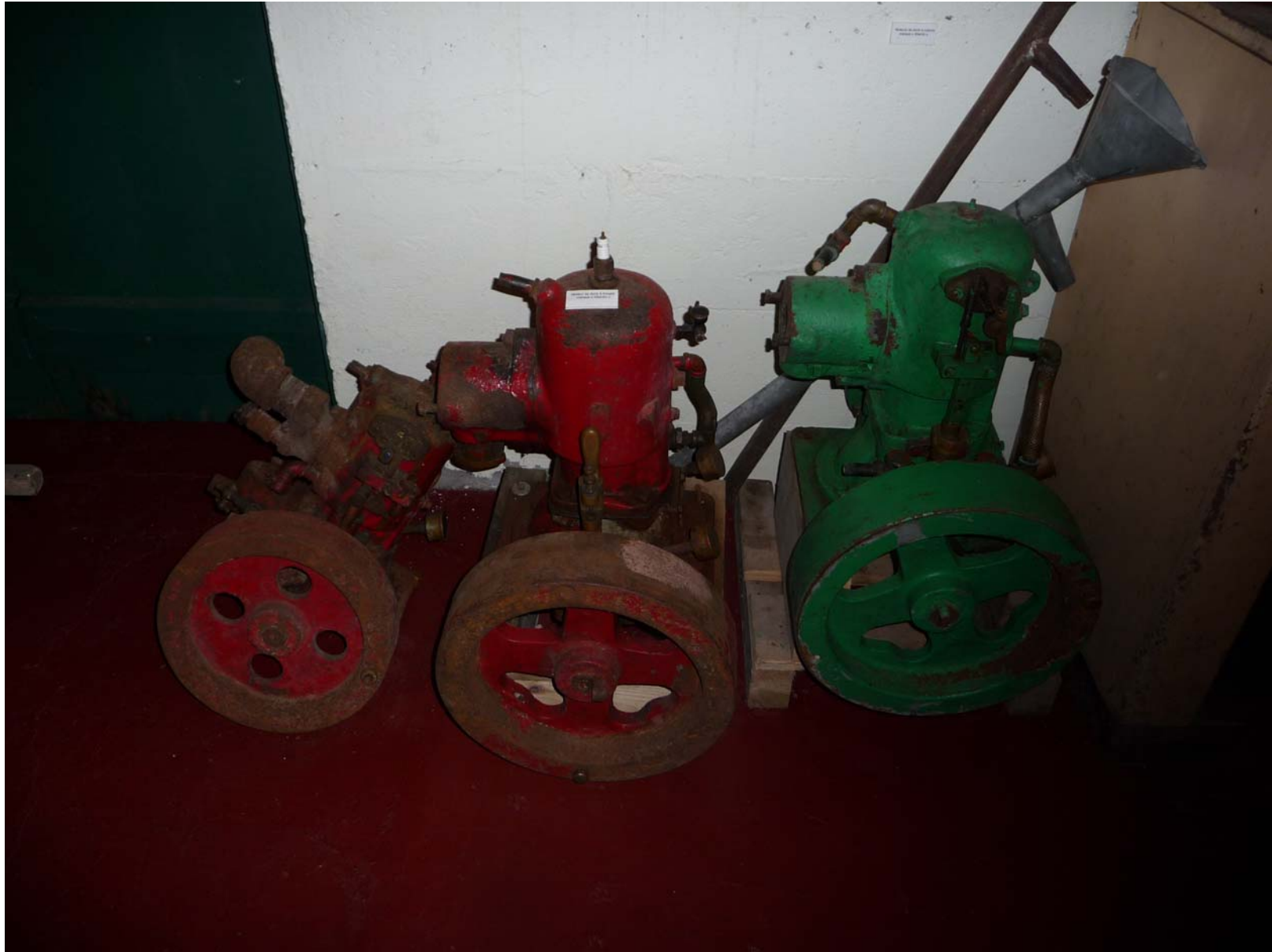
Three “make and break” one-lung (cylinder) engines used in fishing dorys.
