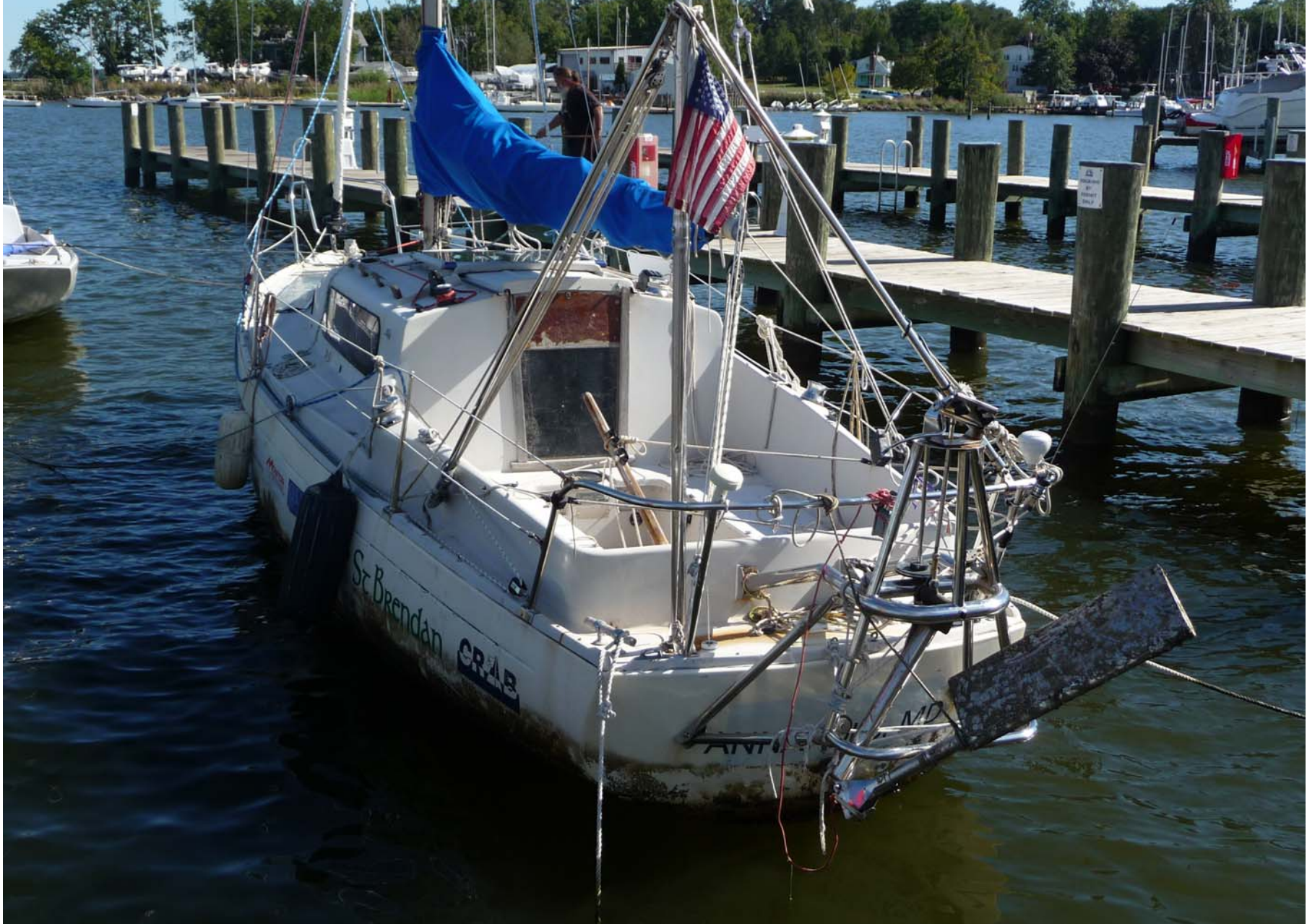
The gel coat on the waterline got wore off by the water action. Barnacles on the self-steering rudder.
